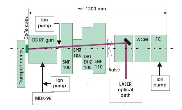
Figure 2: Reduced CTF2 drive beam layout for Pilot test
